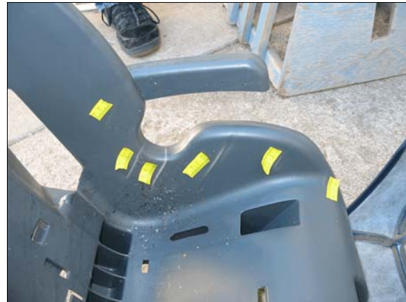
Figure 17: White stress marks in plastic shell of booster seat from deformation of the left side of seat during the crash
