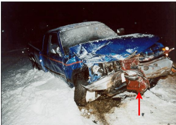
Figure 4: On-scene photo of front damage to Dodge, arrow shows outer sheet metal of case vehicle's driver door stuck to bumper
