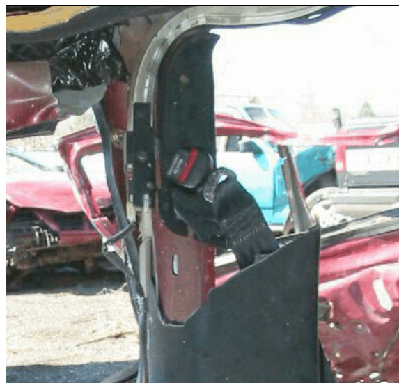
Figure 22: Driver's buckle in B-pillar lock box, automatic shoulder belt in restrained position
