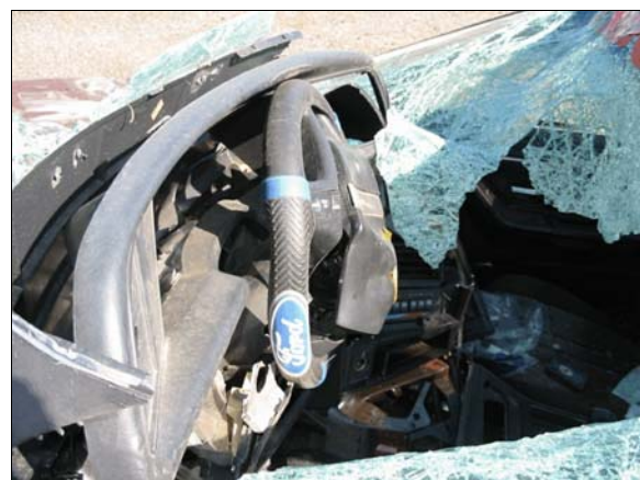
Figure 13: Left side view of deformation to the steering wheel and steering column
