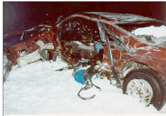
Figure 5: On-scene photo of damage to left side of case vehicle due to impact with the Dodge
