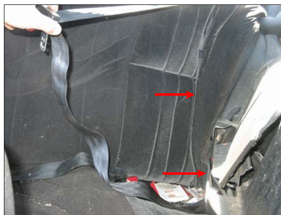
Figure 21: Case vehicle's back left safety belt appeared stretched, arrows show intrusion of seat back and left side panel rear of the B-pillar, view front to rear
