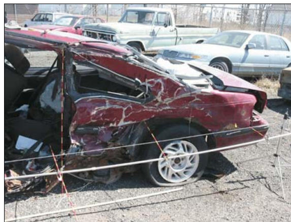
Figure 10: Damage to case vehicle's left quarter panel due to impact with the Dodge
