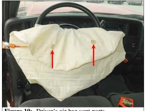
Figure 10: Driver's air bag vent ports
