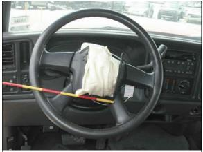
Figure 9: Driver's air bag module flaps
