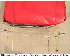
Figure 4: Top view of crush to front of case vehicle
