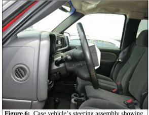
Figure 6: Case vehicle's steering assembly showing lack of deformation
