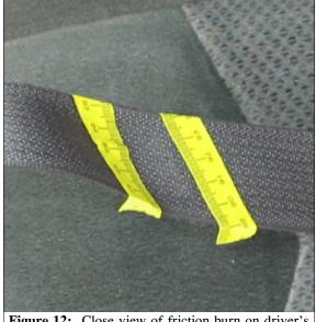
Figure 12: Close view of friction burn on driver's safety belt webbing
