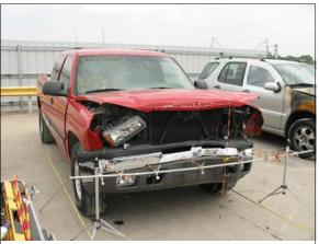
Figure 8: Overview of front damage from front right corner
