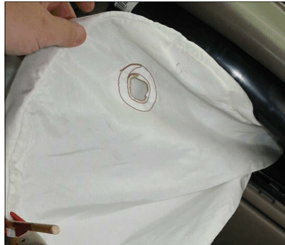
Figure 14: Vent port on right side of case vehicle's front right passenger's air bag
