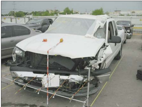
Figure 2: Front damage from impact with the impact attenuator, each increment of tape on hood is tenth of meter, each increment on rods is 5 cm (2 in)
