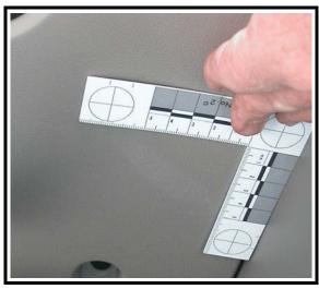
**Figure 10**. Right knee contact to lower instrument panel
