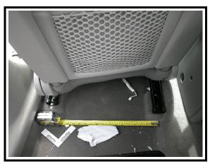
**Figure 7**. Seat movement from seat track failure
