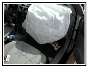
Figure 9. Front right passenger's air bag
