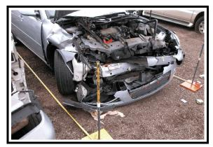
**Figure 5**. Impala frontal damage from impact with truck
