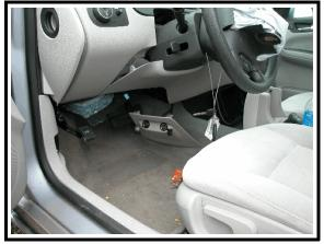
**Figure 13**. Impala lower instrument panel, knee bolster
