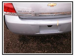
**Figure 6**. Impala rear damage from impact with guardrail
