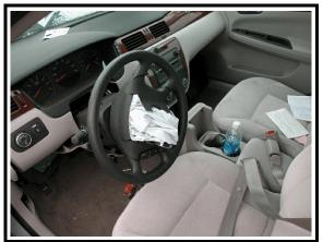
Figure 11. Driver's air bag, module covers
