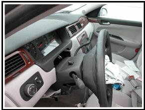
**Figure 7**. Steering column separation (Chevrolet Impala)
