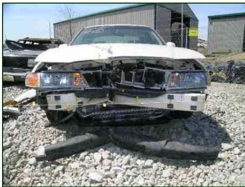
Figure 3. Frontal damage to the Lincoln Continental.
