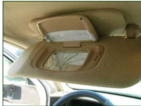
Figure 9. Fractured vanity mirror.
