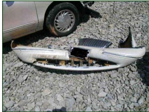
Figure 5. Separated bumper fascia.
