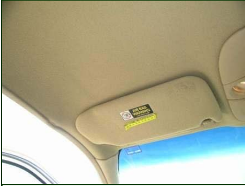
Figure 6. Impacted left sun visor.
