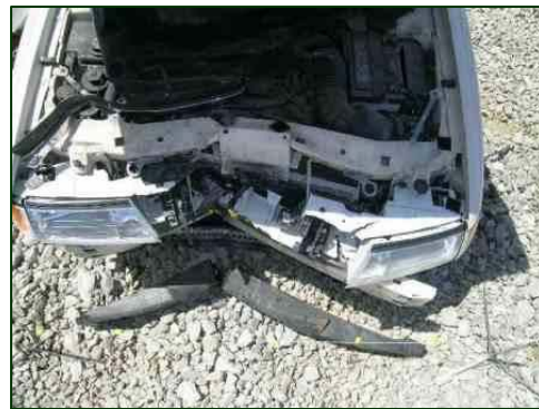
Figure 4. Overhead view documenting the extent of frontal crush.
