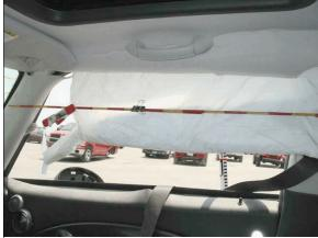
**Figure 12:** Front portion of case vehicle's right side curtain air bag
