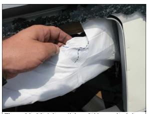
**Figure 14:** Mesh inner lining of side curtain air bag located inside outer nylon bag
