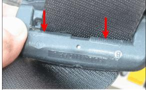
**Figure 16:** Load abrasion on case vehicle driver's latch plate belt guide
