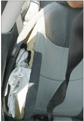
**Figure 10:** Case vehicle's front right passenger seat back-mounted air bag located in right side of seat back
