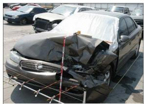
Figure 2: Overview of front damage to Buick from impact with back of case vehicle, vertical scale in tenths of meter, each increment on rods is 5 cm (2 in)
