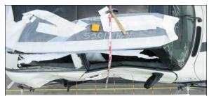
Figure 7: Top view of crush to case vehicle's right front door from impact with back left corner of Subaru
