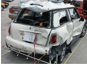
Figure 3: Overview of damage to back of case vehicle from impact with Buick and damage to right front door from impact with Subaru
