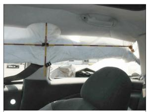
Figure 13: Back portion of case vehicle's right side curtain air bag
