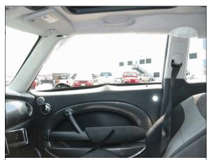
Figure 9: Case vehicle's right front door and side curtain air bag tucked into headliner
