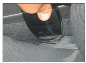
**Figure 17:** Case vehicle driver's safety belt buckle stalk is compressed indicating actuation of pretensioner in crash
