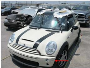
**Figure 5:** Arrow shows damage to front left bumper corner from impact with concrete median barrier
