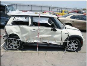
**Figure 4:** Damage to case vehicle's right front door from impact with Subaru and induced damage to right quarter panel from back impact with Buick
