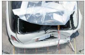
**Figure 6:** Top view of crush to back of case vehicle from impact with Buick
