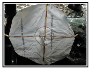
Figure 24. Deployed driver's front air bag
