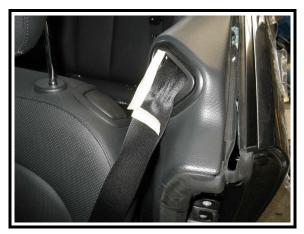
**Figure 17**. Signs of occupant loading to driver's shoulder belt
