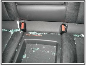
**Figure 22**. Second row seat belt buckle pretensioners activated
