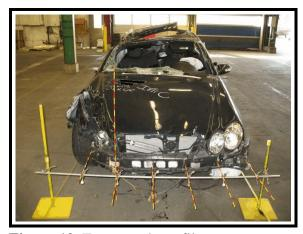
Figure 10. Front crush profile
