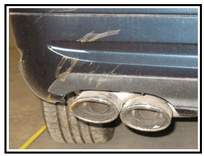
**Figure 15**. Brown transfers from wood marker contacted during the rollover event
