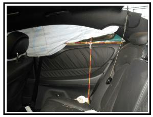
**Figure 26**. Deployed right side curtain - gap at B pillar
