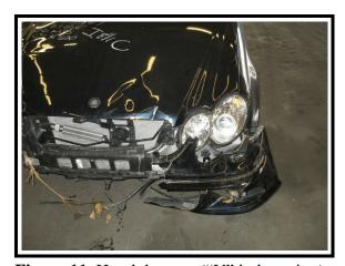
**Figure 11**. Hood damage ("V" indentation) from impact with signpost
