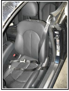
**Figure 20**. Driver's seat belt (cut by fire/rescue)
