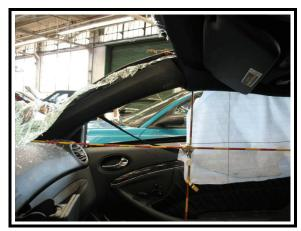
**Figure 25**. Deployed right side curtain - gap at A pillar
