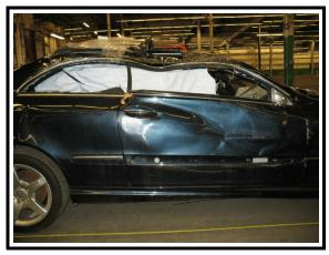
**Figure 14**. Rollover event - vertical and lateral max crush location
