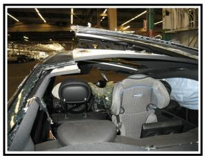
Figure 16. Roof cut by fire/rescue personnel
