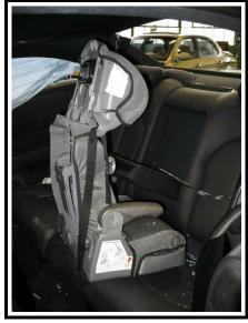
**Figure 30**. Evenflo Big Kid booster seat as found (not secured/not in use during crash)
