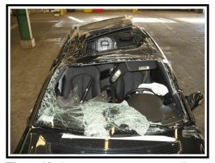
**Figure 13**. Passenger compartment rollover damage
