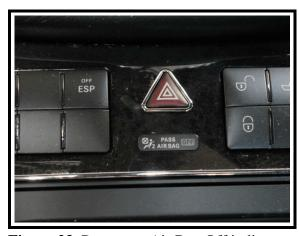
Figure 23. Passenger Air Bag Off indicator
