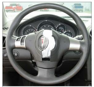
Figure 10: Case vehicle's steering wheel and air bag module cover flaps
