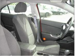
Figure 8: Overview of case vehicle driver's seat as found and left front door, seat is in rear-most position, subsequently determined that driver had seat adjusted to between middle and forward-most position at time of crash
