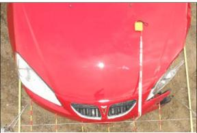
Figure 5: Top view of minimal crush to front of case vehicle, left corner of bumper fascia was torn off from impact with Chevrolet and minimal engagement of case vehicle's bumper bar, each increment on rods in 5 cm (2 in)
