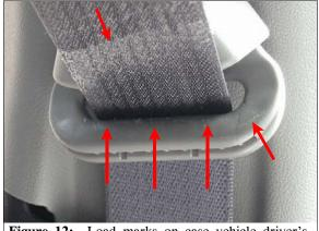
Figure 12: Load marks on case vehicle driver's shoulder belt and "D" ring (arrows)
