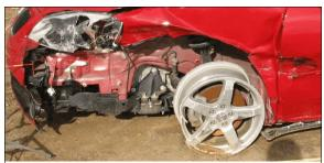
Figure 6: Rearward displacement of case vehicle's left front wheel due to engagement with the Chevrolet's right front corner during impact
