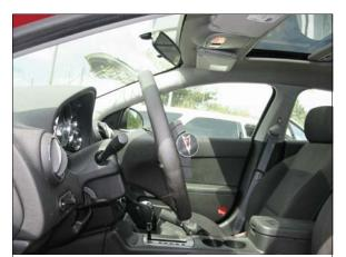
Figure 9: Left side view of steering wheel and steering column showing lack of deformation
