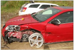
Figure 4: Damage to left fender and displacement of left front wheel from impact with right front corner of Chevrolet.
