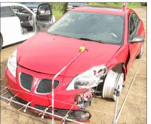
**Figure 3:** Overview of damage to front left corner of case vehicle from impact with right front corner of Chevrolet, increments on tape measure in 10ths of meter, each increment on rods is 5 cm (2 in)
