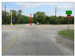
Figure 1: Approach of case vehicle northbound to intersection, red arrow shows area of initial impact, yellow arrow shows area of rollover
