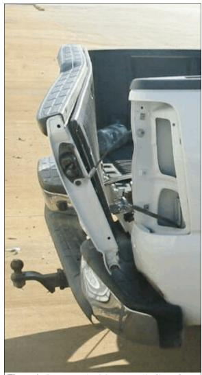
**Figure 4:** Damage to back bumper and tailgate from secondary impact with Ford
