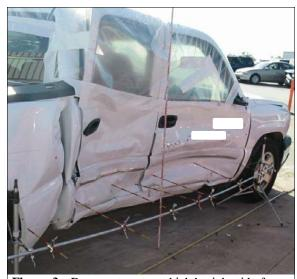
**Figure 3:** Damage to case vehicle's right side from impact with front of Ford
