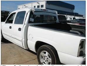
**Figure 5:** Overview of minor rollover damage to left side a case vehicle's cab
