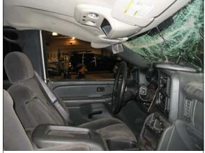
Figure 11: View of Chevrolet driver's seat position, roof intrusion and windshield header intrusion
