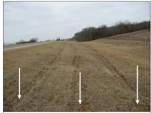
**Figure 3:** Chevrolet's tire marks (left and center arrows) and trailer tire marks (right arrow) in grass approaching rollover location
