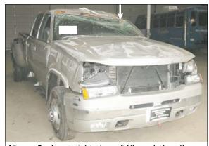
**Figure 5:** Front right view of Chevrolet's rollover damage, arrow shows location of maximum vertical crush to windshield header
