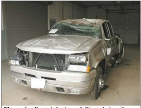
**Figure 6:** Front left view of Chevrolet's rollover damage
