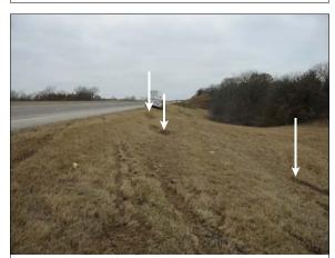
**Figure 4:** Chevrolet's approach to rollover, divots in ground (arrows) show contact of trailer during rollover
