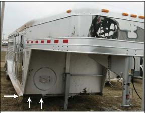
**Figure 9:** Front right view of trailer, arrows show grass jammed in running board and front frame
