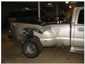
**Figure 8:** Damage to right side of truck bed due to interaction with the trailer during the rollover
