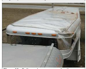
Figure 10: Rollover damage to top of trailer
