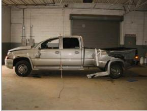
**Figure 7:** Left side view of Chevrolet's rollover damage, damage to truck bed due to interaction with trailer during rollover
