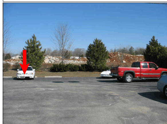
Figure 7: Arrow shows location where target first came into surrogate driver's view as he looked over right shoulder out of backlight; distance back of Chevrolet to target was 7.6 meters (24.9 feet)
