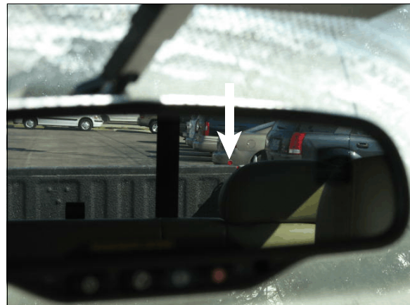
Figure 9: Close view through rearview mirror from driver's seat, arrow shows target where it began to be obstructed by the back right head restraint
