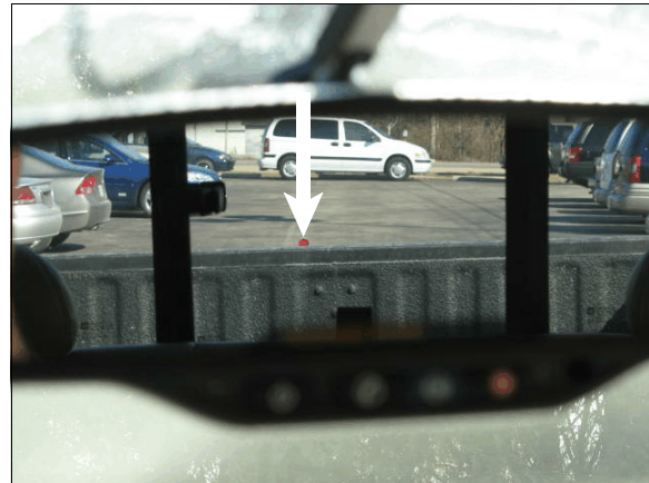
Figure 8: Close view through rearview mirror from driver's seat; arrow shows target at point it first became visible to surrogate driver
