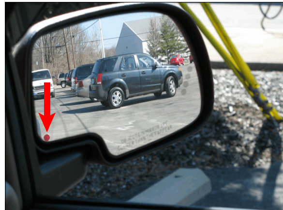
Figure 12: Close view through right side view mirror from driver’s seat; arrow shows target where it first came into driver’s view as it was moved rearward from right rear bumper corner
