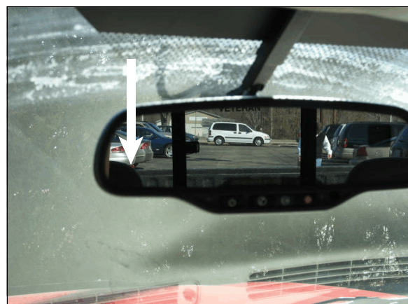
Figure 10: View through rearview mirror from driver's seat; arrow shows target at point it began to be obstructed by the back left head restraint
