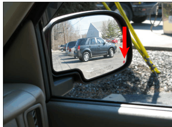
Figure 13: Close view through right side view mirror from driver’s seat; arrow shows target where it begins to go out of mirror’s field of view
