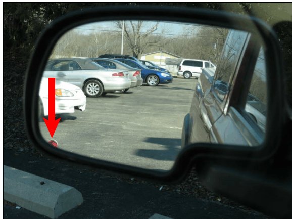
Figure 11: Close view through left side view mirror from driver’s seat; arrow shows target where it began to go out of mirror’s field of view
