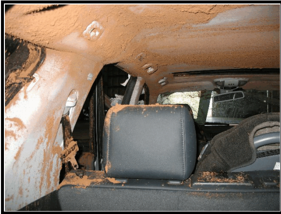
Figure 7. Overview of water/mud damage
