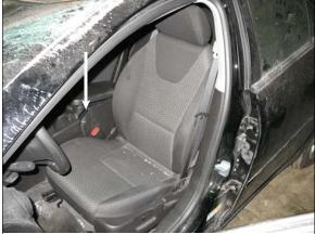
Figure 8: View of driver's seat and broken floor console (arrow)
