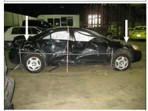
Figure 3: Damage to right side doors from contact with impact attenuator; left arrow shows damage from impact with concrete traffic barrier; right arrow show damage to right fender from the rollover
