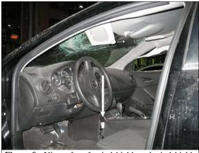
Figure 9: View of roof, windshield, and windshield header intrusion; arrow shows broken console
