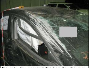
Figure 6: Pavement scratches from the rollover on the right A-pillar
