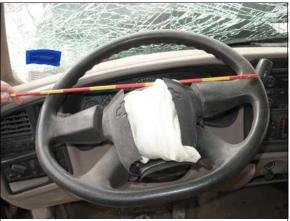
**Figure 10:** Steering wheel damage and air bag flaps
