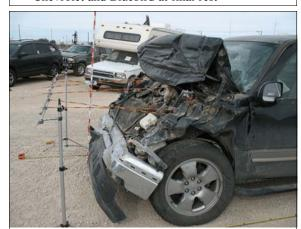
**Figure 7:** Profile of frontal damage measured at upper radiator support level
