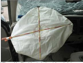
Figure 11: The driver's deployed frontal air bag
