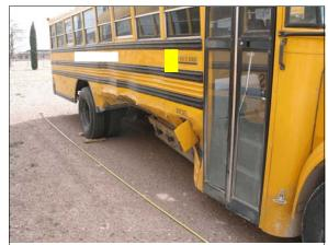
**Figure 5:** Damage to right side of Bluebird from impact with the Chevrolet
