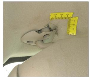
**Figure 9:** Hair embedded in the driver's sunvisor swivel post bracket and contact to the front header
