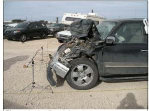
Figure 4: Profile of frontal damage measured at bumper level
