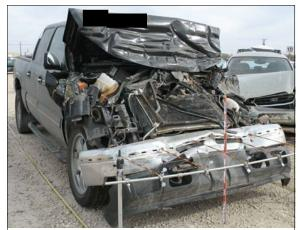
**Figure 1:** The damaged 2007 Chevrolet Silverado C1500 Crew Cab pickup truck
