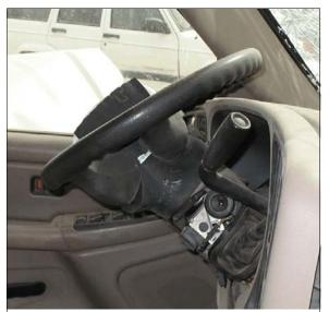
Figure 8: Deformation of the steering wheel and compression of the steering column due to occupant loading
