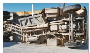
**Figure 12:** Arrow shows fuel tank and fuel tank frame; there was no damage to the tank or fuel leakage
