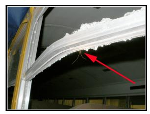
**Figure 10**. Area of ejection, contact evidence on sash
