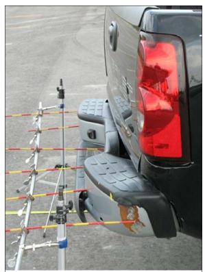
Figure 8: Damage to Chevrolet's back right bumper corner viewed from right
