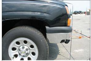
Figure 11: Chevrolet's right front tire restricted by damaged front right bumper corner
