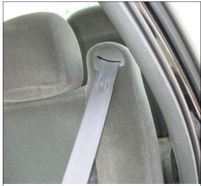
Figure 16: Chevrolet's driver safety belt webbing showing loading evidence (oblique pinch mark and stretching) near should belt guide
