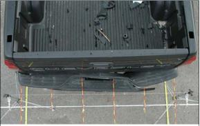
**Figure 9:** Overhead view of Chevrolet's back crush profile with contour gauge set a bumper level
