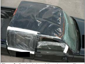
Figure 5: Overhead view of direct damage to Chevrolet's roof from the rollover and induced damage to windshield glazing
