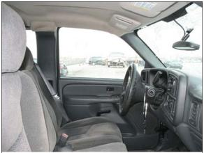
Figure 13: Chevrolet's driver seat area showing undeformed steering wheel rim and inside, windshield-mounted, rearview mirror broken off windshield by impact forces
