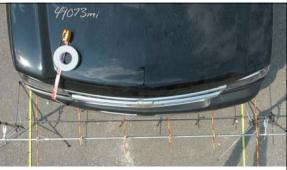
Figure 7: Overhead view of Chevrolet's front crush profile with contour gauge placed at bumper level
