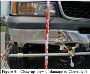
Figure 6: Close-up view of damage to Chevrolet's front right bumper area
