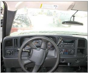
Figure 12: Chevrolet's driver seating area showing no apparent contact evidence on steering wheel, instrument panel, or greenhouse areas and nondeployment of driver's air bag
