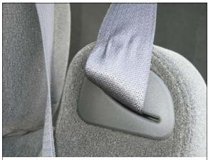
Figure 17: Stretch marks on underneath side Chevrolet's driver safety belt near shoulder belt guide
