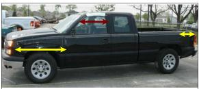
Figure 4: Arrows show areas of damage to the left side from the rollover
