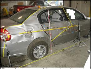
Figure 8: Damage to right side from sideswiping two trees (events 4 and 5)
