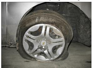
Figure 6: Damage to right front wheel from impact with a rock
