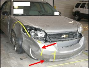
Figure 4: Bottom arrow shows impact location on lower bumper fascia with a rock (event 1), top arrow shows impact location with a tree (event 3)
