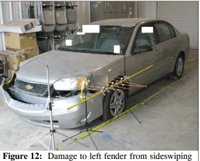
Figure 12: Damage to left fender from sideswiping a tree (event 10)
