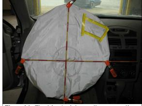
Figure 14: The driver's air bag; yellow tape outlines a dark scuff, but it did not appear to be an occupant contact
