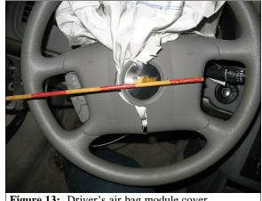
Figure 13: Driver's air bag module cover
