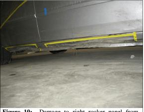
Figure 10: Damage to right rocker panel from impact with a rock (event 7)
