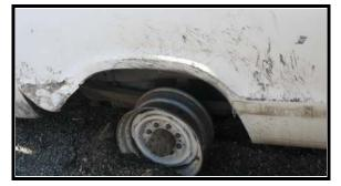
Figure 9. Tire-related right rear damage
