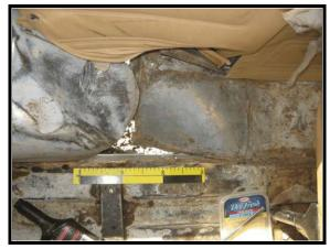
**Figure 10**. Torn area of wheel well (right of row 4)
