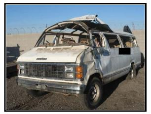
Figure 8. Rollover damage, subject vehicle
