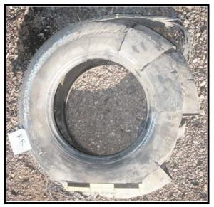
Figure 6. Right rear tire (outboard aspect)
