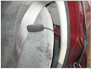
Figure 10: Shoulder belt clip attached to elastic tether cord for second row left seat belt
