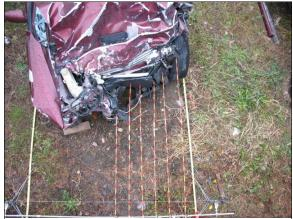
Figure 7: Overhead view of Chevrolet's front crush profile
