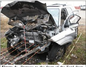
Figure 4: Damage to the front of the Ford from impact with the front of the Chevrolet
