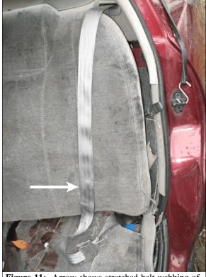
Figure 11: Arrow shows stretched belt webbing of second row left seat belt
