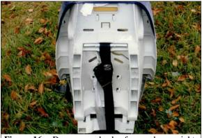
Figure 16: Damage on back of second row right CSS
