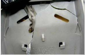
Figure 17: Close view of damage to the shell of the second row right CSS
