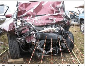
Figure 6: Damage to front plane of the Chevrolet from the impact with the front of the Ford
