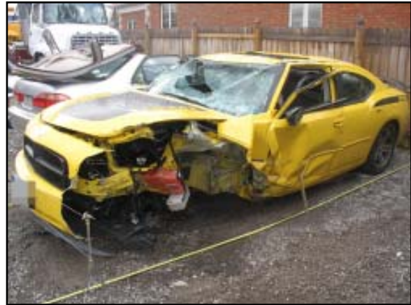
Figure 6: Direct contact damage extending down left side of the Dodge.
