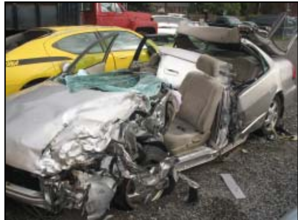
Figure 10: Residual left side damage to the Honda.
