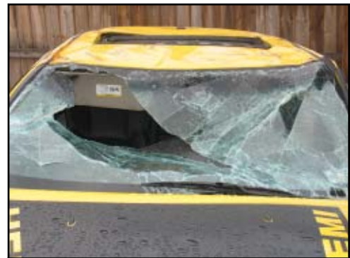
Figure 7: Image depicting the maximum vertical roof crush at the windshield header of the Dodge.
