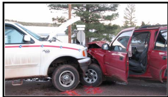
Figure 3. Frontal damage to Isuzu (police photo)
