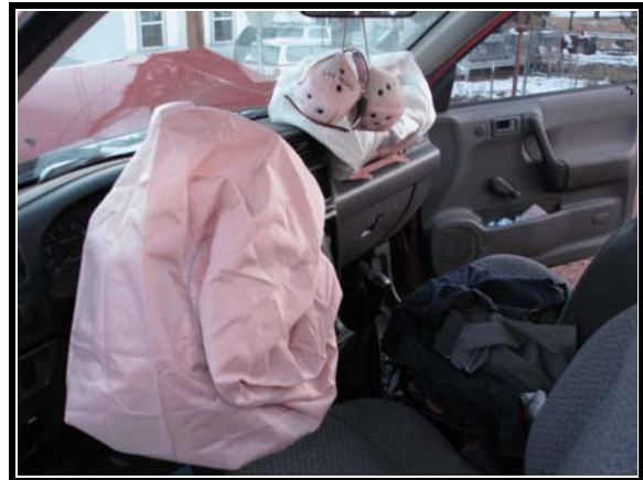
Figure 4. Driver and front right passenger air bags (police photo)
