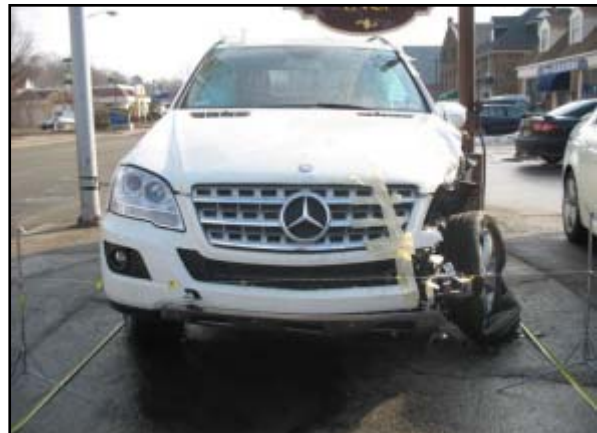
Figure 4. Residual frontal damage from the tree impact.
