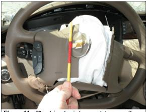
**Figure 11:** The driver's air bag module cover flaps
