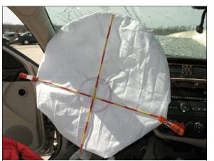
Figure 12: The driver's deployed frontal air bag
