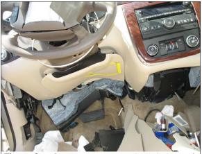
Figure 8: Occupant contact to knee bolster of Chevrolet
