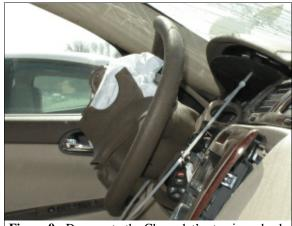
Figure 9: Damage to the Chevrolet's steering wheel due to loading by the driver
