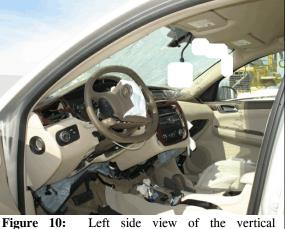
Figure 10: Left side view of the vertical displacement of the instrument panel and steering assembly
