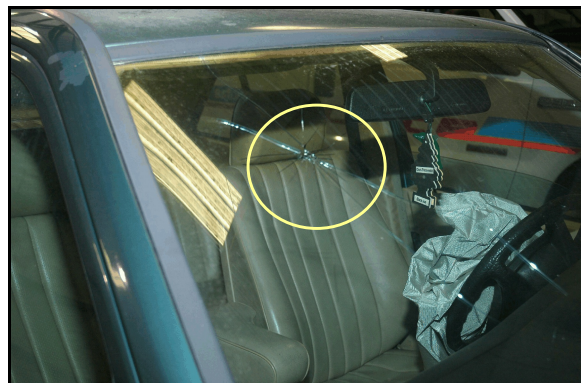
Figure 4: Star-shaped crack in the Mercedes' windshield, confirmed as pre-existing damage
