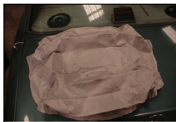
Figure 8: Driver's air bag fabric, front portion, after disassembly of the air bag module
