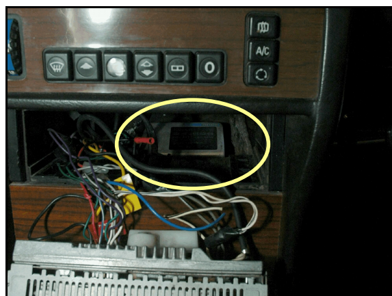
Figure 6: Access to the SRS control module, behind the radio in the center instrument panel console
