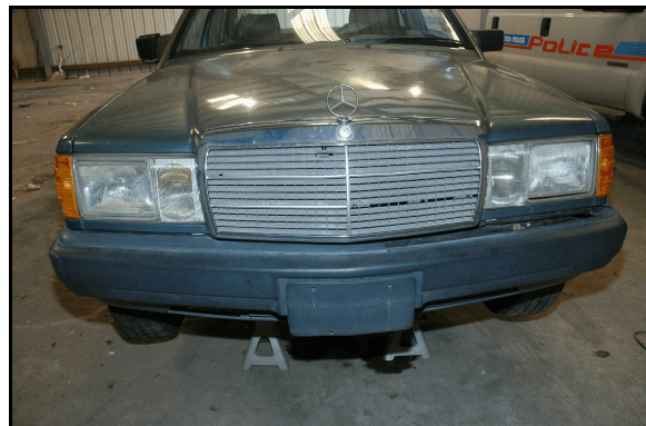
Figure 3: Entire front of the Mercedes at impound facility; note, absence of frontal impact damage
