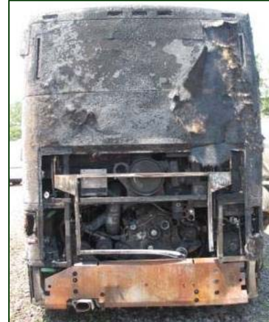
Figure 8. Fire damage to the back of the motorcoach.
