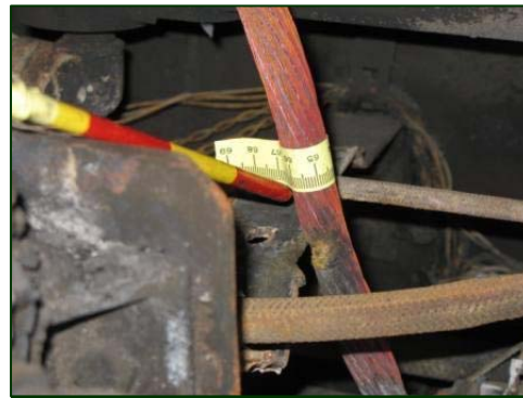
Figure 17. Arced starter cable against bracket.
