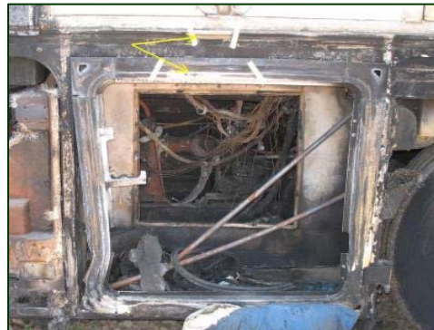
Figure 11. High heat oxidation to the area above the right side engine compartment door.
