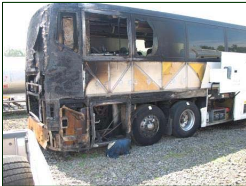
Figure 10. Fire damage to the right rear side area of the motorcoach.
