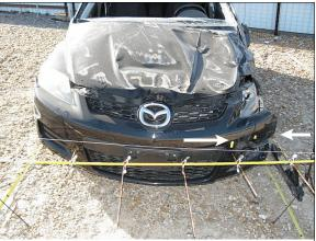
Figure 4: Arrows show the damage on the front bumper from the impact with the Jeep
