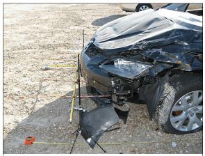
Figure 8: Left side view of the impact area on the left portion of the front bumper
