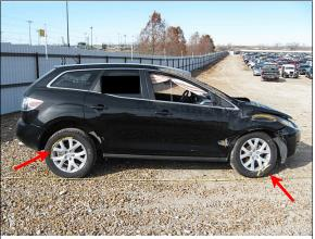
Figure 5: Arrows show the damage on the right front and right rear wheels from the curb impacts
