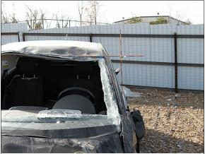
Figure 14: The maximum vertical crush occurred on the windshield header
