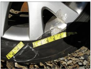
Figure 10: Damage to the right front rim and tire from the curb impact
