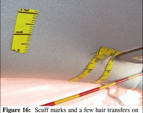
Figure 16: Scutt marks and a few hair transfers on the left roof side rail and adjacent roof
