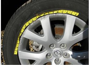
Figure 11: Damage on the right rear rim from the curb impact
