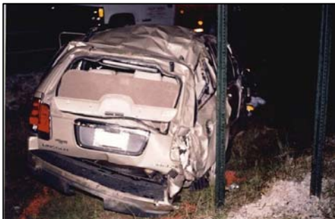
Figure 8. Damage to the back plane of the Lincoln.
