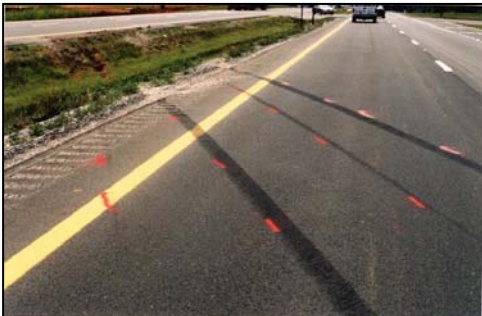
Figure 4. CCW rotation of the Lincoln off the south shoulder to the trip point.
