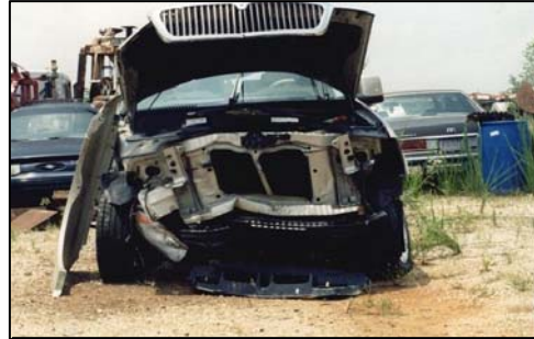
Figure 7. Left lateral displacement of the frontal structure.
