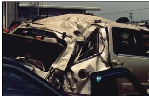
Figure 9. Close-up view of the crush to the right D-pillar area.
