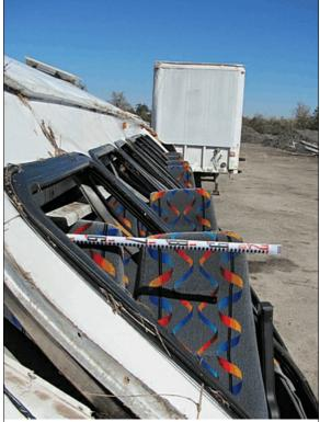
Figure 14: Front to rear view of the right shift of the roof and status of the outboard seats
