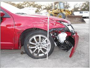
**Figure 4:** Damage on right side of the Mercury from impact with the left side of the Ford; vertical scale in 10<sup>th</sup> of meter
