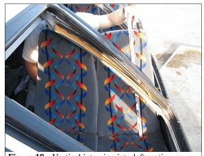
Figure 18: Vertical intrusion into left seating rows
