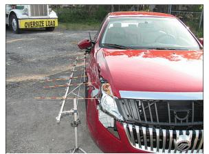
Figure 22: Crush on the right fender of the Mercury
