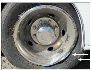
**Figure 7:** Arrows show black rubber transfer on the rim and contact on the left rear tire of the Ford from engagement with the right front wheel of the Mercury
