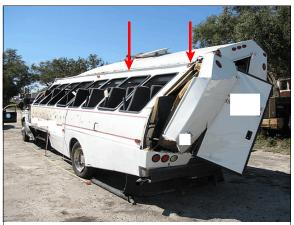
Figure 11: Arrows show location of pavement abrasions on the left roof side rail and roof; grass and dirt were entrapped in the roof side rail forward of this area
