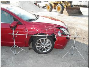
Figure 21: Damage on the right fender and right front wheel of the Mercury from the impact with the left side plane of the Ford
