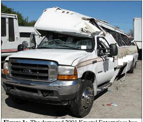
Figure 1: The damaged 2001 Krystal Enterprises bus
