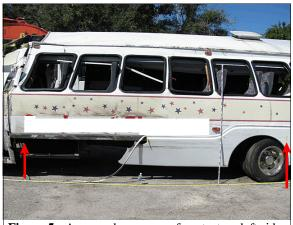
Figure 5: Arrows shows area of contact on left side of the bus from the impact with the Mercury; arrow on right shows extent of red paint transfer
