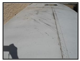
**Figure 12**. Roof damage (looking toward front of bus)
