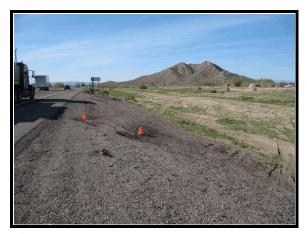
**Figure 5**. Rear bus tire trip points. Right side road departure.
