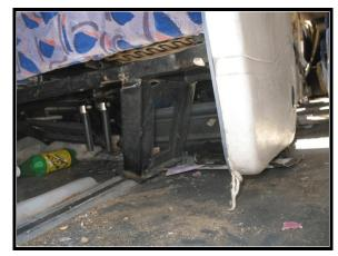
**Figure 13**. Exemplar shifting of inboard seat leg
