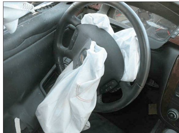
Figure 9: The driver's frontal air bag did not fully deploy
