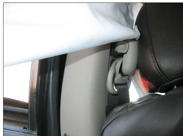
Figure 12: The deployment of the left IC air bag was obstructed when the intrusion of the left B-pillar closed the gap between the B-pillar and the seat back
