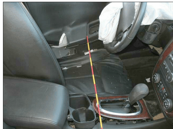
Figure 6: Intrusion of the left front door of the Chevrolet into the driver’s seat position
