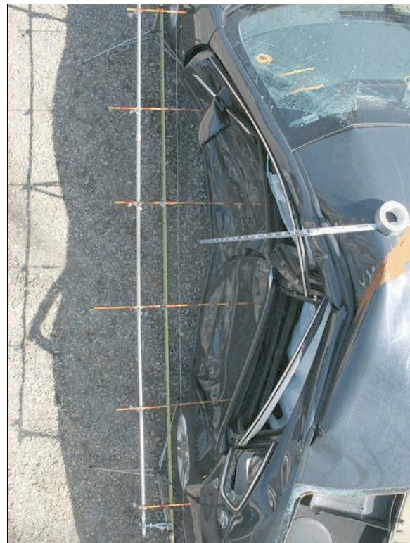
Figure 5: The crush on the left side of the Impala from the impact with the front of the Jeep
