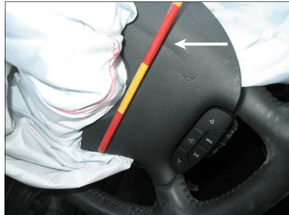
Figure 8: The top seam on the right air bag module cover flap did not separate (arrow)
