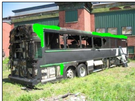
Figure 8. Right side fire damage to the motorcoach.
