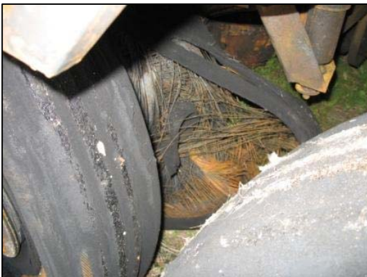
Figure 16. Remains of the left inner drive axle tire.
