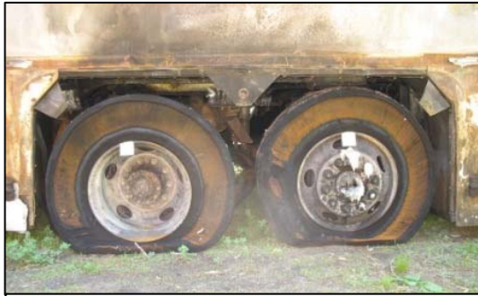
Figure 11. Fire damage to the left drive and tag axle tires.
