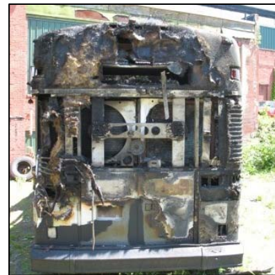
Figure 6. Fire damage to the back of the motorcoach.
