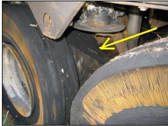
Figure 12. Remains of the left inner drive axle tire (arrow).
