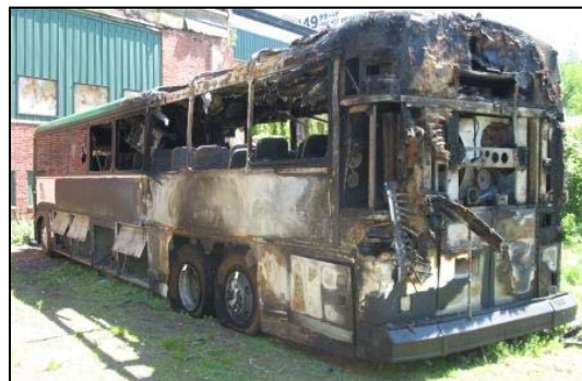
Figure 10. Glazing damage to the left side of the motorcoach.
