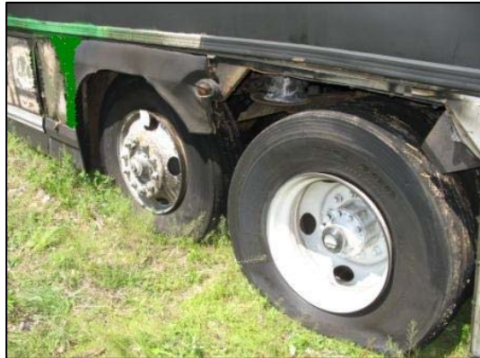
Figure 13. Right drive and tag axle tire damage.
