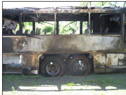
Figure 17. High heat damage above the left drive and tag axle locations.
