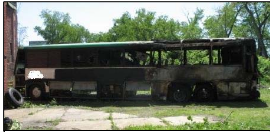
Figure 5. Left side view of the fire damage to the motorcoach.
