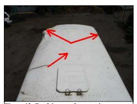
Figure 12: Roof damage from towing activities.
