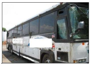
Figure 15: Rear view of the right side glazing status.
