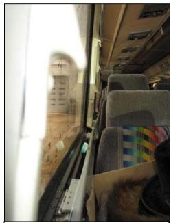
Figure 13: Rear view of the lateral intrusions along the right side of the interior.
