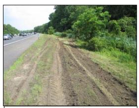
Figure 7: Trajectory and CCW yaw of the motorcoach across the roadside slope.
