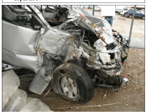
Figure 3: Damage on the front right bumper corner and right fender from the impact with the 18 cm (7.1 in) diameter metal streetlight pole
