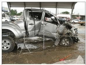
Figure 7: Damage on the right side doors from the impact with the 33 cm (13 in) diameter wood utility pole
