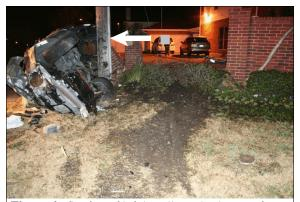
Figure 6: Section of brick wall was broken out from impact with vehicle's front plane; divot on ground shows touchdown location of left side plane of vehicle; arrow shows utility pole impacted by right side plane (Police image, view south)
