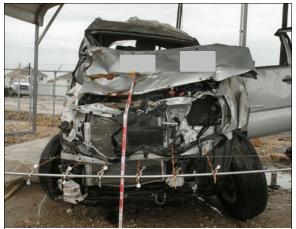
Figure 5: Damage on the front plane from the brick wall impact overlapped the damage on the front right corner from the metal streetlight pole impact
