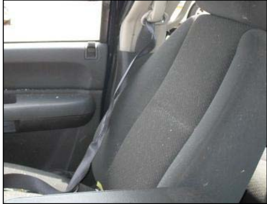
Figure 8: Abrasion to the right front webbing from contact with head restraint posts.
