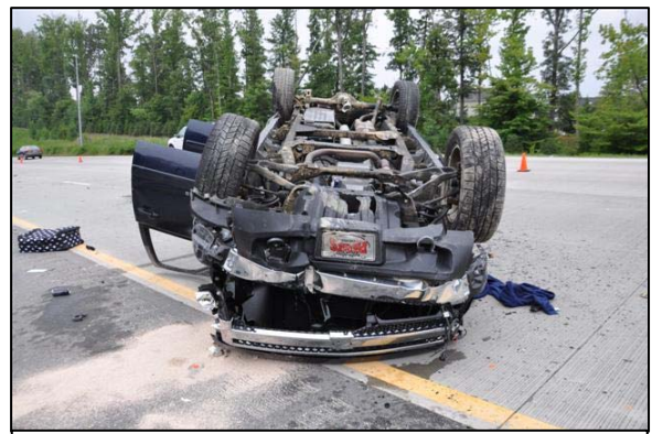
Figure 6: View of the Chevrolet at final rest taken by the police investigator depicting the undercarriage damage.
