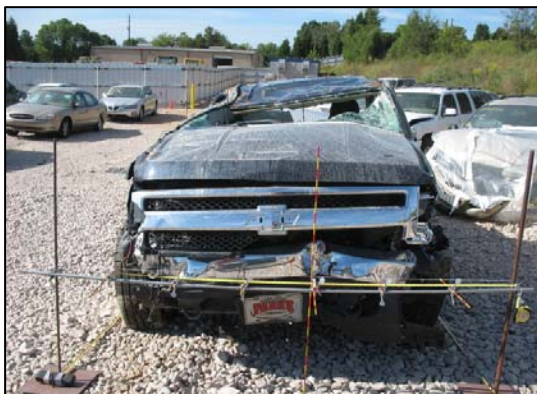
Figure 5: Frontal damage to the Chevrolet taken during the SCI inspection.
