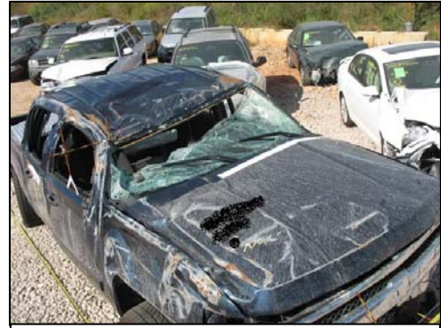
Figure 7: Rollover damage to the top plane of the Chevrolet.
