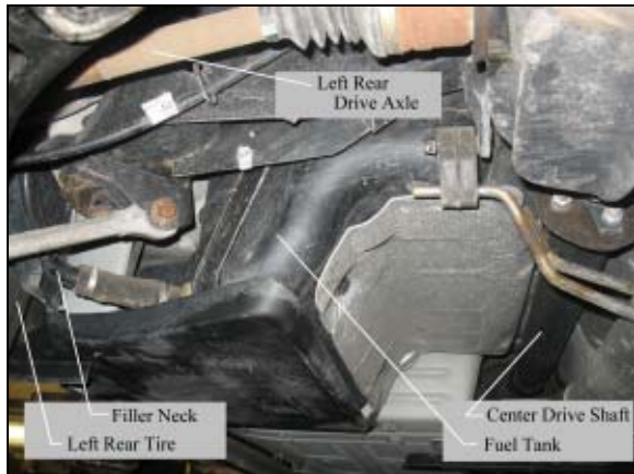
Figure 5: View depicting the orientation of the undercarriage of an exemplar Dodge Charger.
