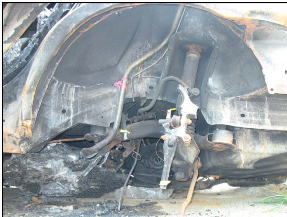
Figure 10: View of the Dodge's left rear wheel well opening and reconstructed position of the filler neck.
