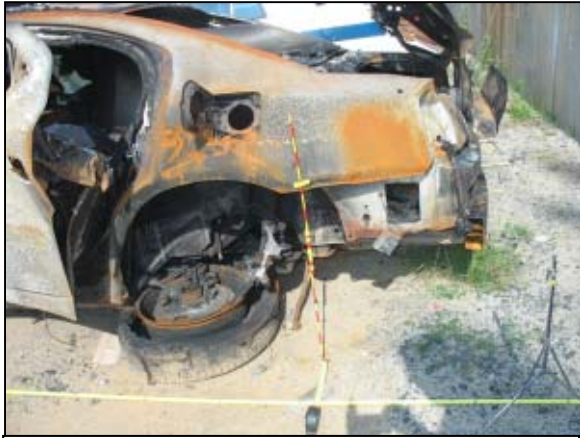
Figure 7: View of the left rear quarterpanel and impact damage to the Dodge.
