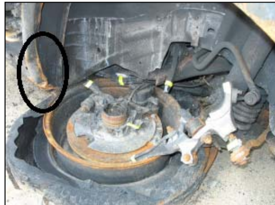
Figure 9: View of the Dodge's fractured rear suspension, bearing casting and separated left rear wheel.
