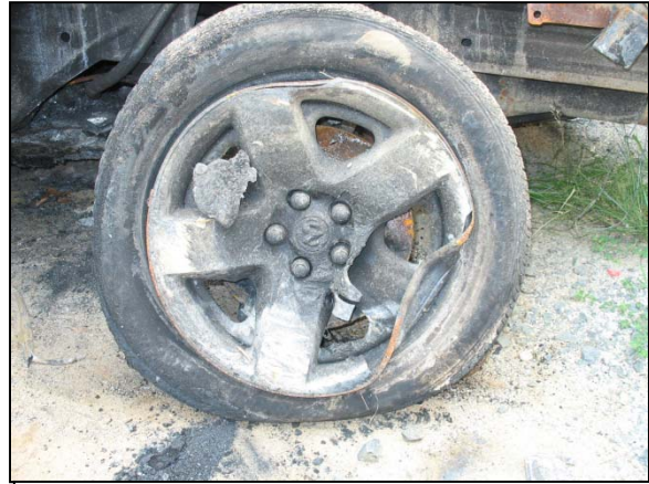
Figure 8: View depicting the damage to the left rear wheel rim of the Dodge.
