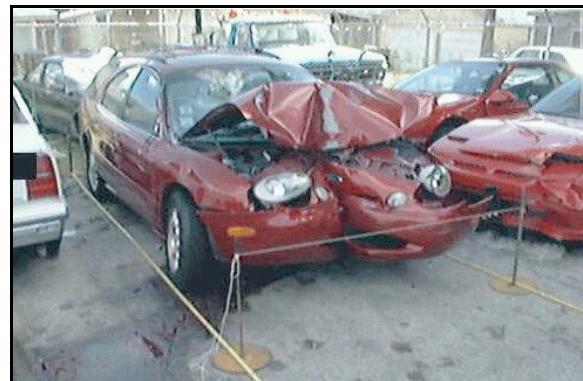
Figure 4: Case vehicle's right side and damaged front from signal pole impact; Note: unknown damage exists on right side
