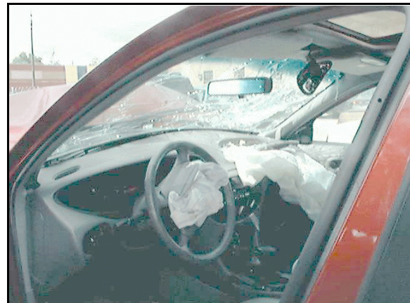
Figure 5: Case vehicle's front seating area from left showing deployed driver and front right passenger air bags
