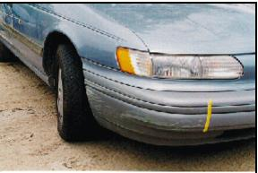
**Figure 10:** Scraping to the case vehicle's front right bumper corner from contacting regulatory SPEED LIMIT sign (3<sup>RD</sup> event) prior to coming to rest (case photo #30)
