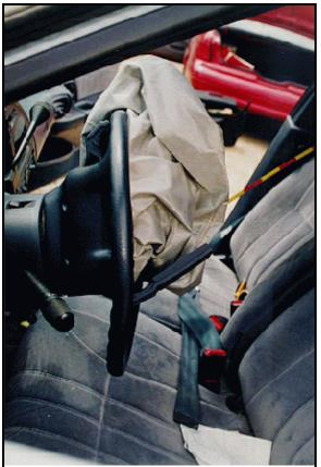
Figure 11: Deformation to top of case vehicle's steer-ing wheel rim which resulted when the driver loaded the deploying air bag causing the air bag to expand backwards into the rim; Note: steering wheel inverted (case photo #34)
