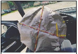
Figure 12: Case vehicle's driver air bag with steering wheel in upright position; Note: yellow tape high-lights area of contact (i.e., skin transfer) by front center passenger (case photo #37)
