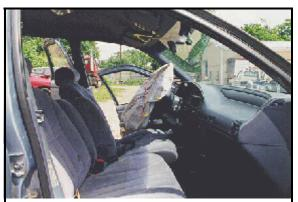
Figure 14: Case vehicle's front seating area; Note: difference in seat track placement between driver and passenger seats, and ceiling tape indicates air bag exhaust residue (case photo #50)
