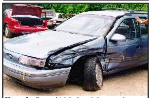
Figure 2: Case vehicle's front left corner damage from impact with vehicle #2; Note: damage extends down left side to driver's door, and vertical yellow tape indicates direct damage length (case photo #20)
