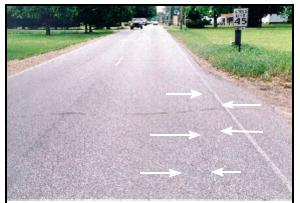
Figure 5: Case vehicle's path of travel after impacting vehicles #2 and #3 showing scuff marks from left front tire (highlighted by arrows) and replaced SPEED LIMIT sign struck before coming to rest (case photo #05)
