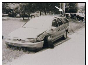
Figure 7: On-scene view of case vehicle at final rest; Note: vehicle #3 (Suburban) in background and struck speed limit sign directly behind case vehicle (case photo #15)
