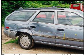
Figure 9: Sideswipe damage to case vehicle's right side from vehicle #3's front left bumper corner (case photo #27)
