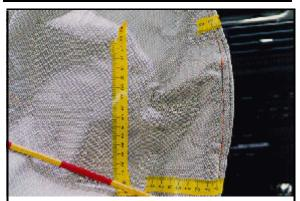
Figure 13: Close-up of skin transfer to right side of case vehicle's driver air bag from contact with the left side of the front center passenger's face (case photo #38)
