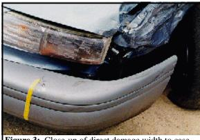
Figure 3: Close-up of direct damage width to case vehicle's front left bumper corner (case photo #23)
