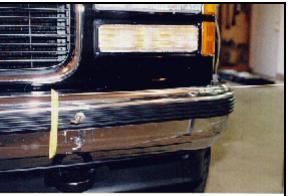
**Figure 17:** Close-up of end swipe damage to vehicle #3's front bumper; Note: missing front left bumper guard (case photo #62)
