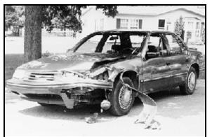
Figure 4: On-scene view of vehicle #2 at final rest showing crush to front left (case photo #54A)
