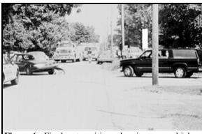
**Figure 6:** Final rest positions showing case vehicle in center background on south roadside, vehicle #2 at left after rotating counterclockwise, and vehicle #3 at right after rotating clockwise (case photo #17)
