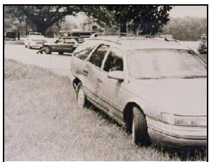
Figure 8: On-scene view of case vehicle's right side damage from end swipe with vehicle #3; Note: vehicle #2 at final rest in background (case photo #16)
