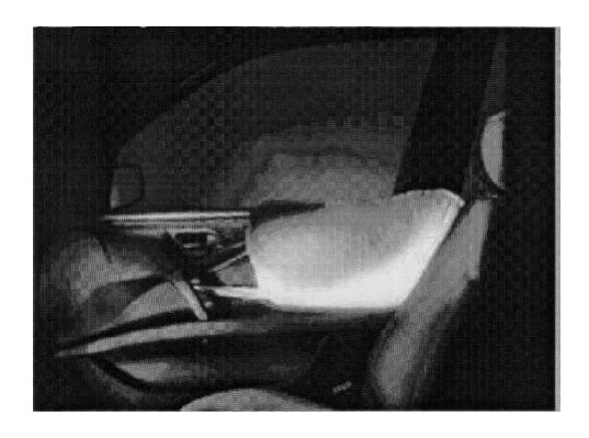
Figure 1. Exemplar photograph of a Mercedes-Benz's deployed doormounted side impact air bag
