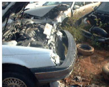
Figure 2. Right lateral view of the crush damage to the upper radiator support of the Ford Taurus.
