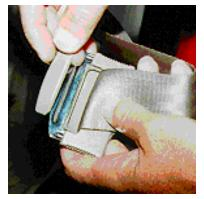
Figure 13. Disjoined plastic binding on the left front latchplate
