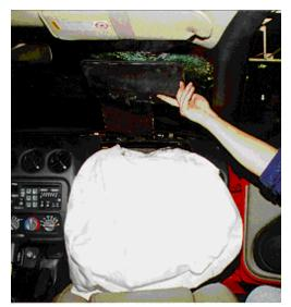
Figure 10. View of the passenger compartment with deployed air bag and air bag module cover flap extended to the damaged windshield
