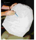
**Figure 7**. Front left air bag of the Firebird with highlighted grey vinyl transfer
