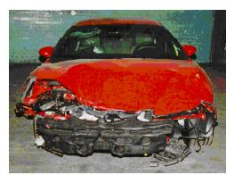
**Figure 1.** View of the damaged frontal plane of the 1998 Pontiac Firebird
