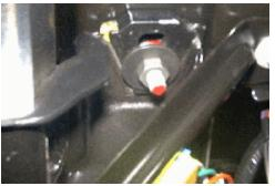
Figure 9. Right side shear capsule showing no movement
