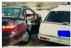
**Figure 1:** Case vehicle's right side damage viewed from approximately 20 degrees right of back
