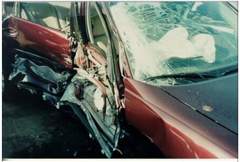
Figure 3: Close-up of case vehicle's right passenger compartment damage viewed from front
