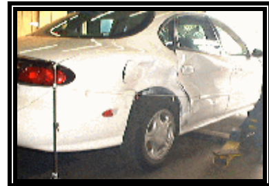
Figure 5. Sideslap damage to the right rear side of the Taurus.
