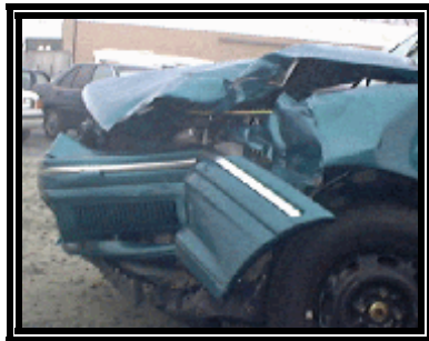
Figure 6. Initial impact damage to the left front side area of the Mercury Tracer.
