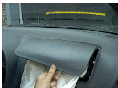
Figure 7- View of the front right air bag module cover
