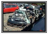
Figure 3. Frontal damage to the 1998 Ford Taurus SE.
