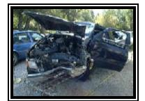
Figure 5. Frontal damage to the 1994 Ford Ranger XL.
