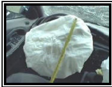
Figure 6. 1998 Ford Taurus SE redesigned driver air bag.
