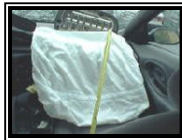
Figure 7. 1998 Ford Taurus SE redesigned passenger air bag.
