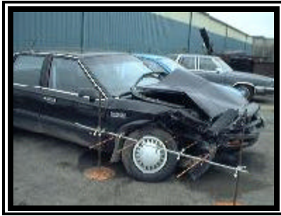
Figure 4. Front right damage to the 1990 Oldsmobile Cutlass Ciera.
