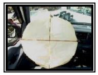
Figure 5. 1999 Ford F-250 pickup truck redesigned driver air bag.
