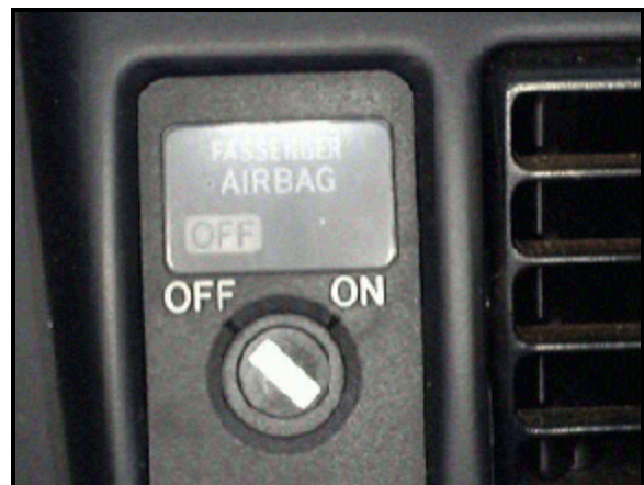
Figure 8. Interior, case vehicle. Passenger air bag shut off switch.
