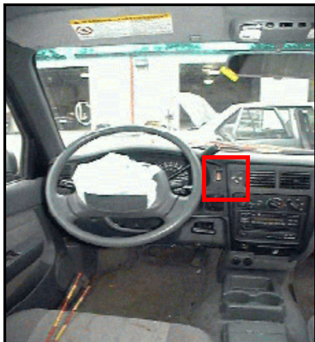
Figure 7. Interior, case vehicle. Box indicates location of air bag shut off switch.
