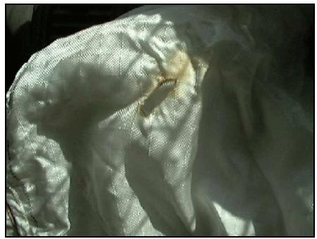
Figure 8. Interior, case vehicle. Passenger's side air bag (burn hole).
