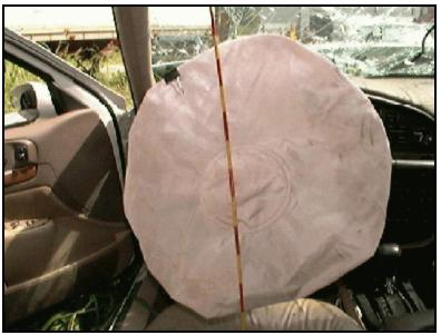
Figure 6. Interior, case vehicle. Driver's side air bag.
