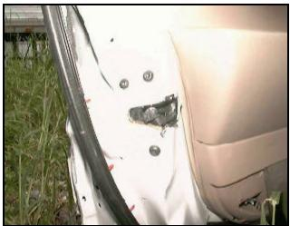
Figure 9. Latch/striker failure, left front door.
